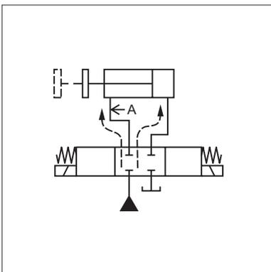
The cylinder may be self-propelled in very slow speed due to leakage at a directional control valve in a circuit as shown in the figure to the left where the load to the cylinder is light and the pressure within the line is retained.
