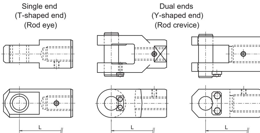
Figure: Example of end bracket
