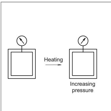
Heating hydraulic fluid within an airtight container will expand the fluid and increase the pressure.
