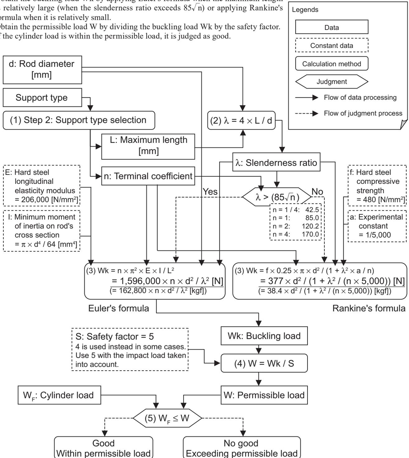
Figure: Flow of buckling calculation
